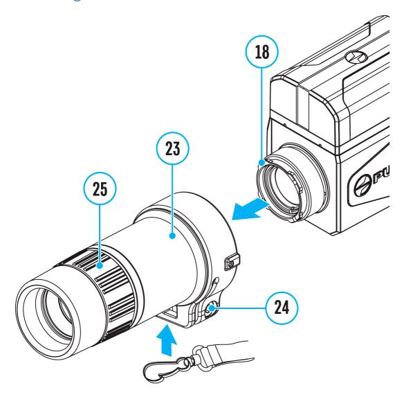
The **Pulsar 3x20 B monocular (23)** (available separately) allows you to transform the attachment into a hand-held thermal imager with 3x magnification.
